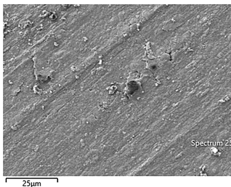
Figure 5. “Spot NO. 25” within the scorched position on the Ti sheet after 30 days of exposure in H 2 where six new elements, i.e., Si, Fe, Al, Ca, Ni, S were detected using EDS.
