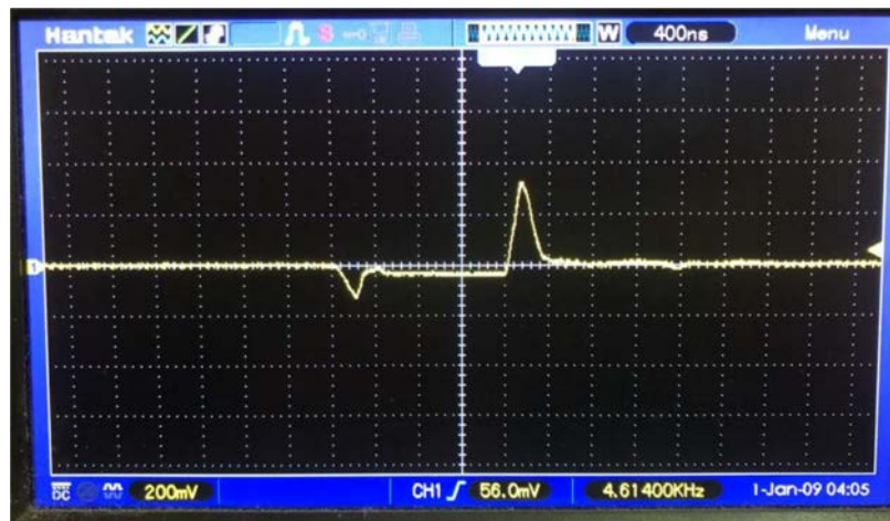
Figure 6. Details of the voltage pulses.
