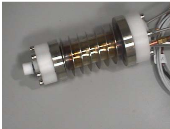
Figure 3 A view of the glow-discharge cell. The channels between the spiraling fins are for coolant flow
