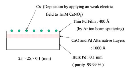
Figure 1. Sample fabricated by MHI
