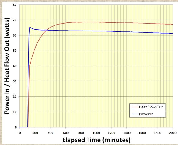
Input power is a near-instant measurement, but output heat flow measure is delayed by long calorimeter time constant
