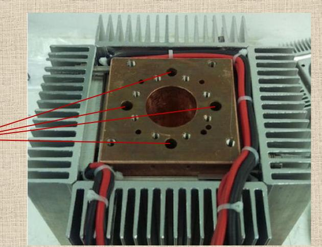
Cartridge heaters + LT discharge + LENR XP (if any) are primary sources of heat in the system.
