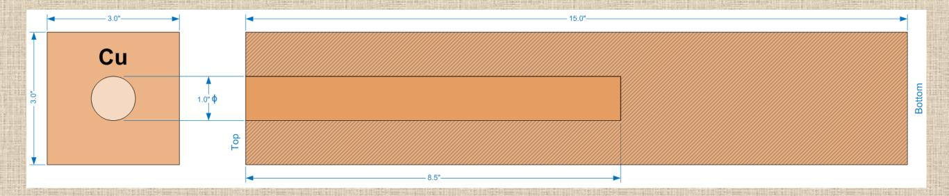
Volume = 2103 cm<sup>3</sup>, mass = 18.8 kg Thermal capacity for  $Cu = 0.385 \text{ J/g-}^{\circ}\text{C}$ Thermal capacity of block = 7254 J/ $^{\circ}\text{C}$
