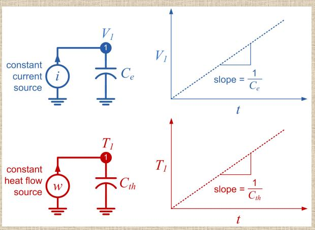
Circuit voltage nodes (state variables) become temp. nodes (also state variables)
