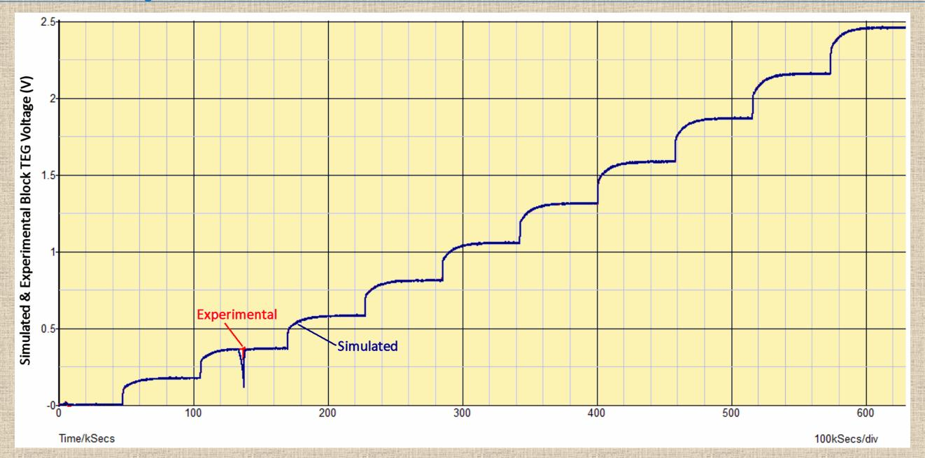
Fast rise exists on each of the stairsteps. This means that two modes are present, not a TEG nonlinearity as suggested by the TEG mfgr.
