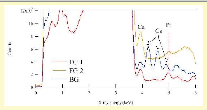
Detection of Pr using SOR X-ray at Spring-8, Harima, Japan (FG1, FG2: Signals from Samples after D2 Permeation
