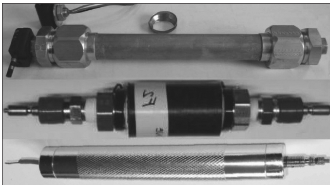
Figure 2. Three generations of the exterior housing for interior Fusion Diode tubes: Mark III (top), Mark IV (middle) and Mark V (bottom).
