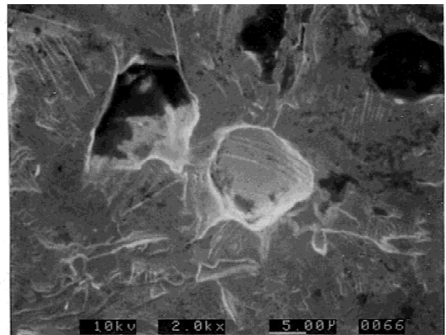
Fig. 8. SEM of a postelectrolysis Pd surface showing the exposed terrace along the fault and holes.
