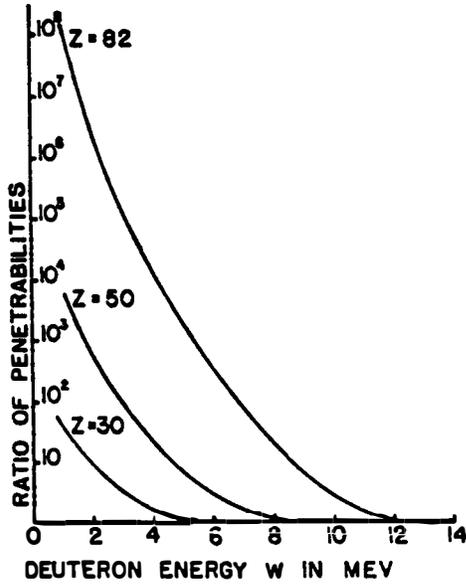
Fig. 1. The ratio of the Oppenheimer-Phillips to the Gamow penetrability of the nucleus potential barrier for different values of the atomic number  $Z$  as a function of the deuteron energy  $W$ , as reported by Volkoff.<sup>16</sup>
