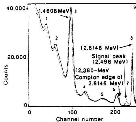
Fig. 6. Gamma-ray spectrum in the Fleischmann and Pons experiments<sup>18</sup> as recalibrated by Petrasso et al.,<sup>19</sup> showing the 7 to 9 peaks beyond the 6 Tl-208 peak.
