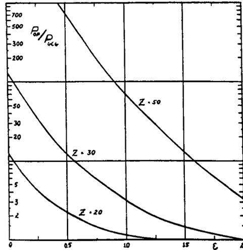
Fig. 2. The ratio of the Oppenheimer-Phillips to the Gamow penetrability of the nucleus potential barrier for different values of the atomic number  $Z$  as a function of the ratio of deuteron kinetic energy to its binding energy, as reported by Bethe.<sup>17</sup>
