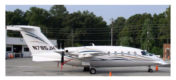
A Piaggio P180 Avanti. The company claims, "The Avanti was developed by discarding conventional aeronautical thinking!" - <a href="http://www.piaggioamerica.com/">http://www.piaggioamerica.com/</a>, but ironically this design is reminiscent of history's first airplanes, the 1903 – 1909 Wright Flyers, with a canard wing forward and twin pusher propellers mounted on the wings. Photo by J. Rothwell
