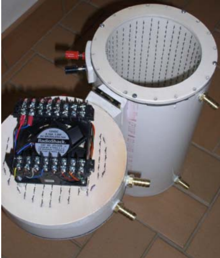
FIGURE 16. Photo of a homemade Seebeck calorimeter based on use of thermocouples. A total of 1000 Type J wire thermocouples were placed in the thermal wall made of PVC tubing. The wires were butt welded on the inside and lead soldered on the outside. The outside surface was waterproofed so that constant temperature water could flow in the surrounding jacket. A muffin fan circulates air within the calorimeter when the lid is closed.
