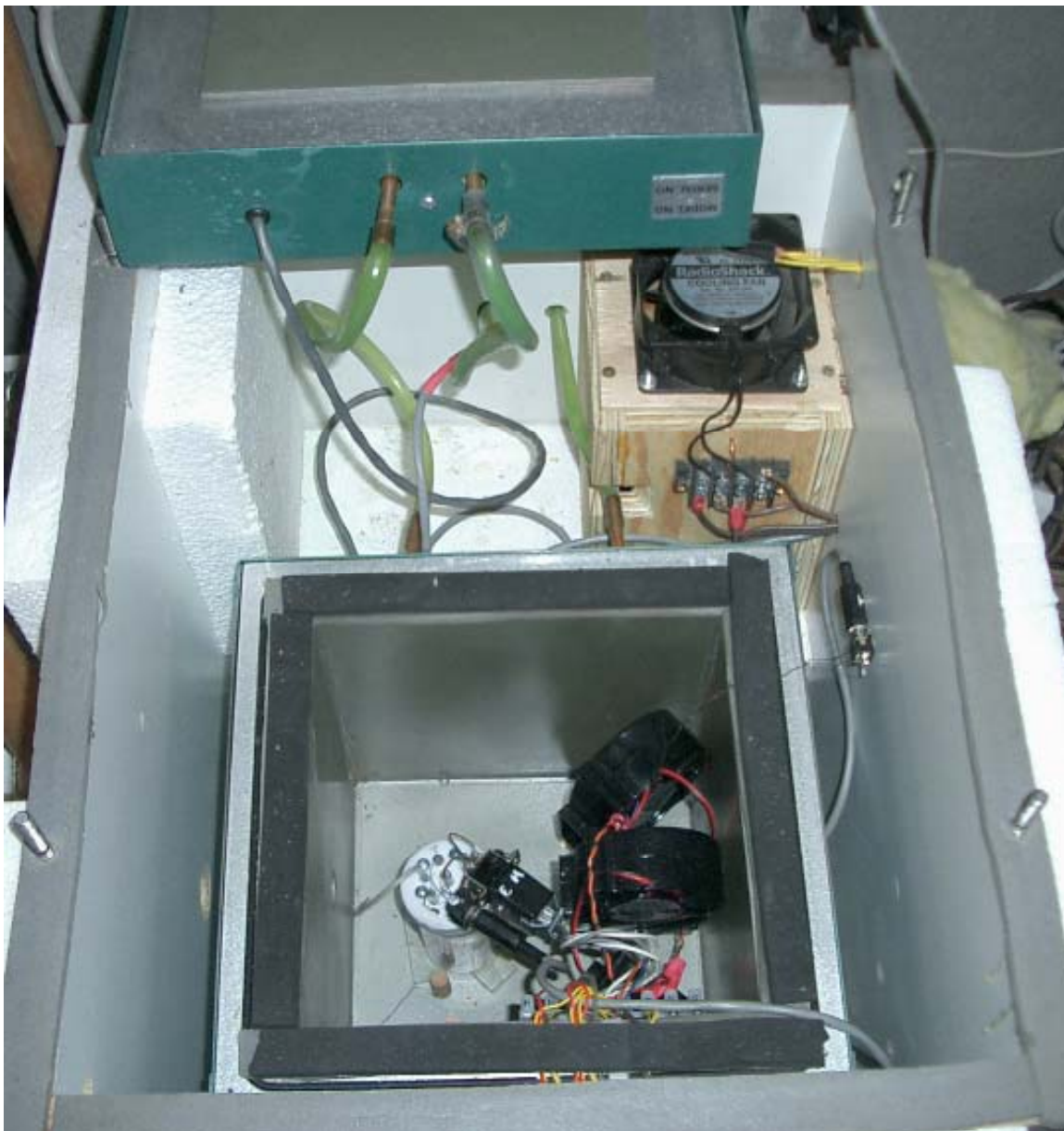
FIGURE 15. Picture of a Thermonetics Seebeck calorimeter 3 . The active enclosure contains three fans and is closed by the green lid sitting off to the back. After the Seebeck is closed, the surrounding box is closed by another lid, which allows the environment to be maintained at the same temperature ( 20^{\circ}\pm 0.02^{\circ} ) as the cooling water provided to the Seebeck enclosure.
