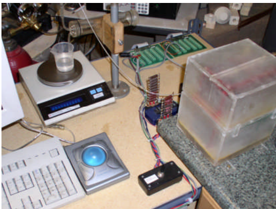
Figure 5. View of calorimeter and oil reservoir for measuring D/Pd ratio. The switch in the foreground allows change from electrolysis to calibration. Water is circulated using a pumped (1.5 l/min) constant temperature bath ( \pm 0.01^\circ\text{C} ).
