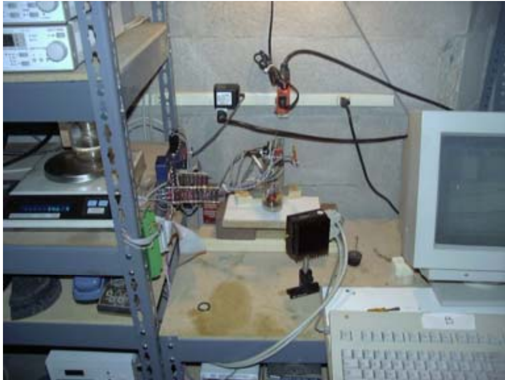
FIGURE 1. Picture of isoperibolic calorimeter before addition of stirrer.
