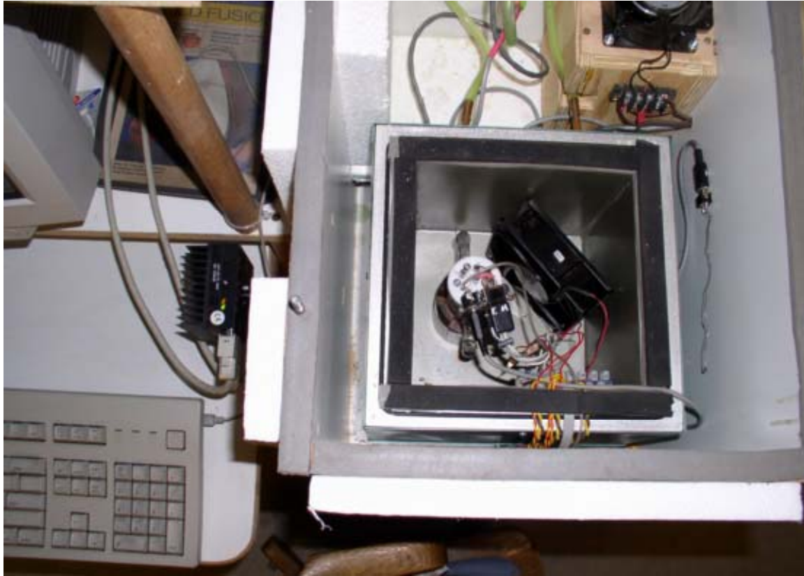
FIGURE 4. Interior view of the Seebeck calorimeter. The Seebeck box is located in a wooden enclosure that is held at \pm 0.02^\circ\text{C} . Only one fan is used in this design.
