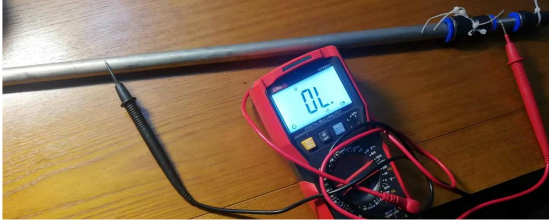
Fig. 8 The inner and outer tubes are checked for electrical isolation..
