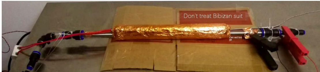
Figure 2. Titanium tube reactor with heater and thermocouple.
