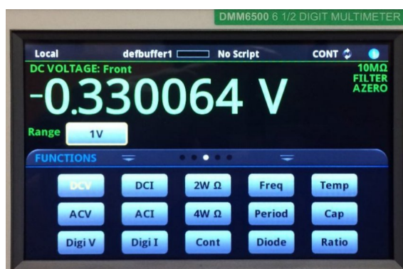
Figure 6. Open circuit voltage measured on the brass - brass device after about 1 hour from the co-deposition and device assembly.
