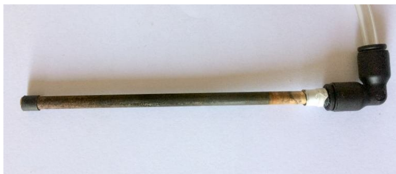
Figure 10. Oxidation appearing on the WE after exposure to air (oxidation is mainly on the left side).
