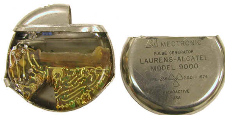
Figure 7. A plutonium powered pacemaker. The plutonium has been removed; it fit into the slot on the top left. See technical details at: https://www.orau.org/health-physics-museum/collection/miscellaneous/pacemaker.html .
