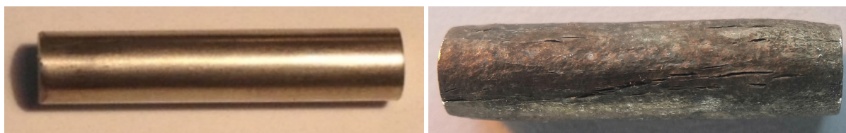
Figure 1. Pd-0.25wt.%B rod from M. H. Miles. (left) new sample; (right) the sample after electrolysis for 2,147 h (89.5 d).
