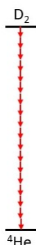
Figure 4. Schematic of naive scheme in which the fusion transition down-converts the nuclear energy to vibrational energy.
