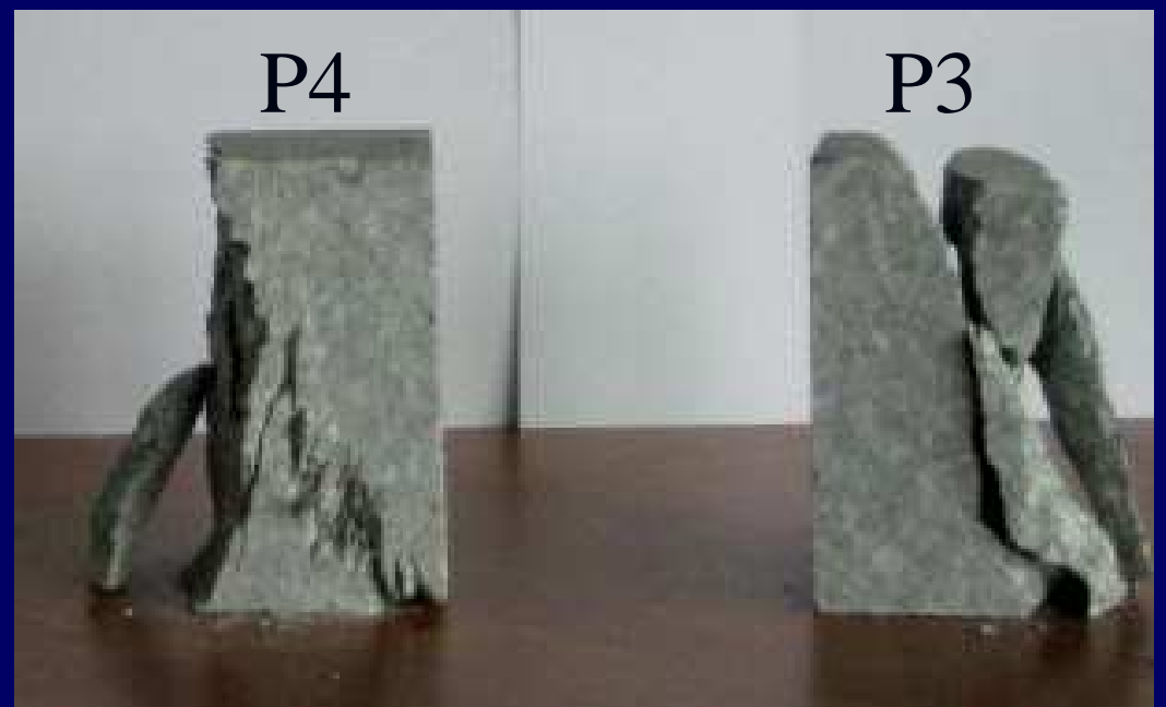
Specimens P3 e P4 in Luserna granite following compression failure.
