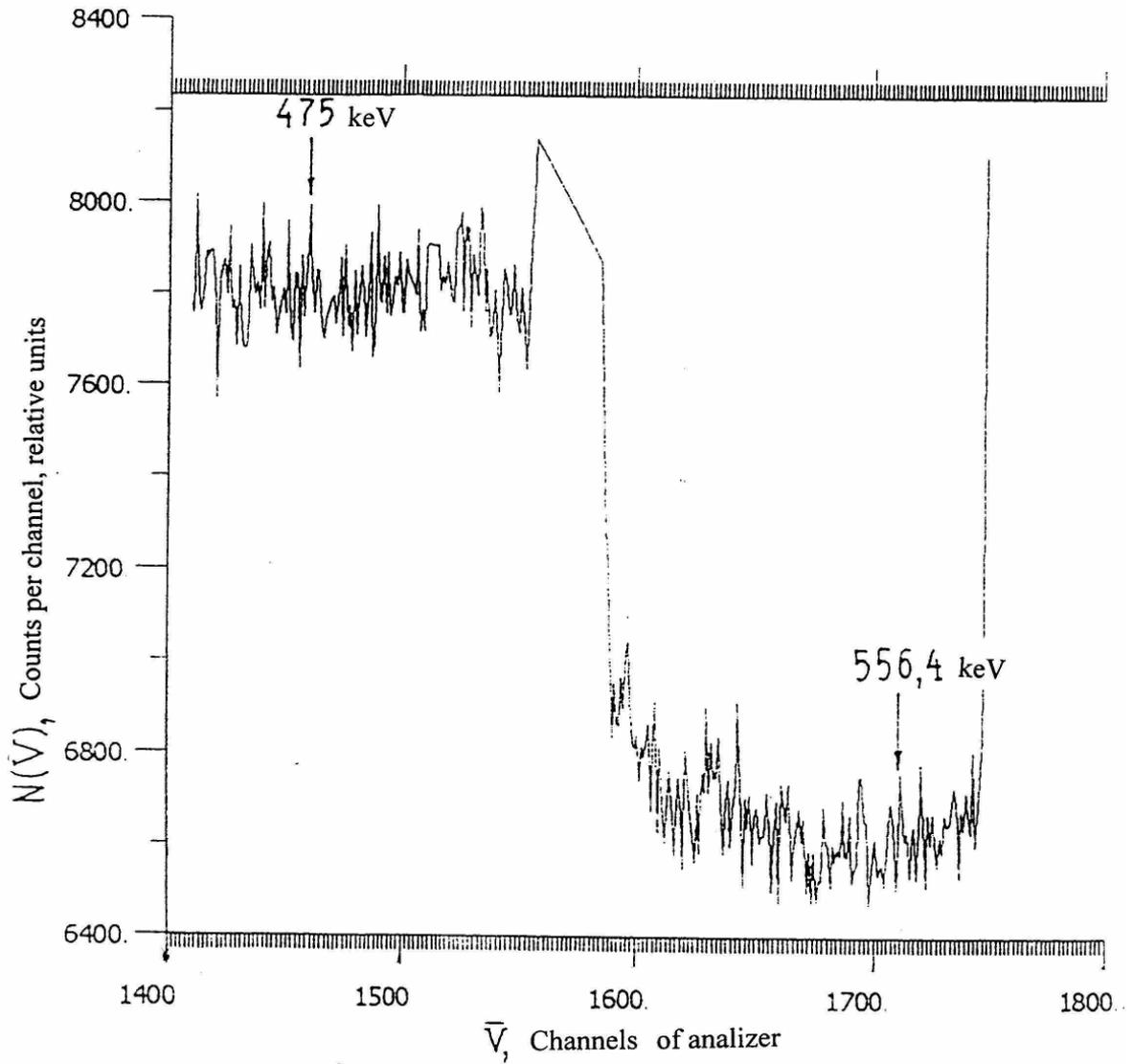
Fig.2. Instrumental spectra of gamma-quanta in the vicinity of the energies of identification of  ${}_{45}\text{Rh}^{102}$  :  $E=475.1$  keV (38.4 quanta per 100 decays) and  $E=556.41$  keV (96 quanta per 100 decays)
