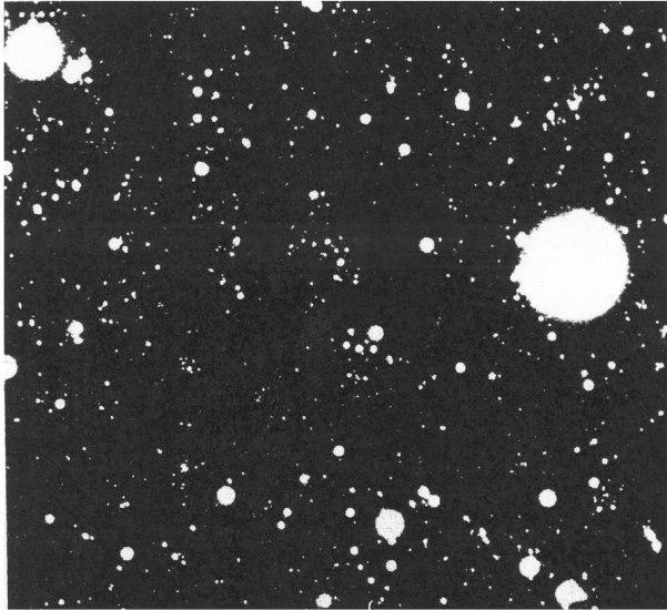
Fig. 7. Photo of gamma beams on an X-ray film with a 2 mm lead screen.
