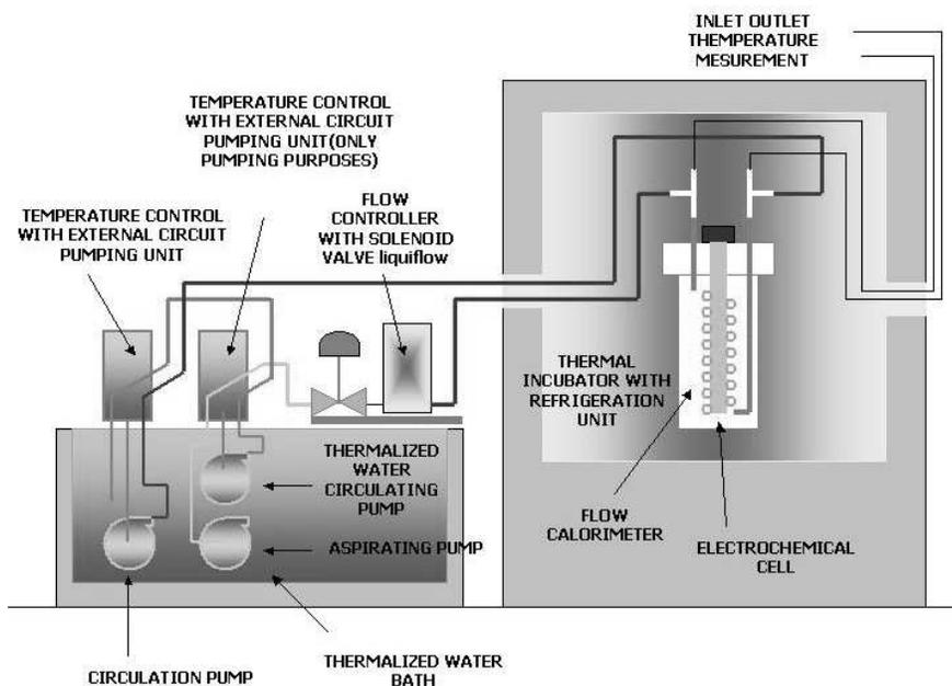
Fig. 2. Flow calorimeter system with electrochemical cell.
