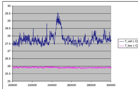
Fig. 7. Electrolyte temperature evolution: the temperature increase is well correlated with excess power.
