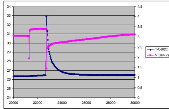
Fig. 9. Electrolyte temperature increasing and voltage evolution during excess power in experiment L30.
