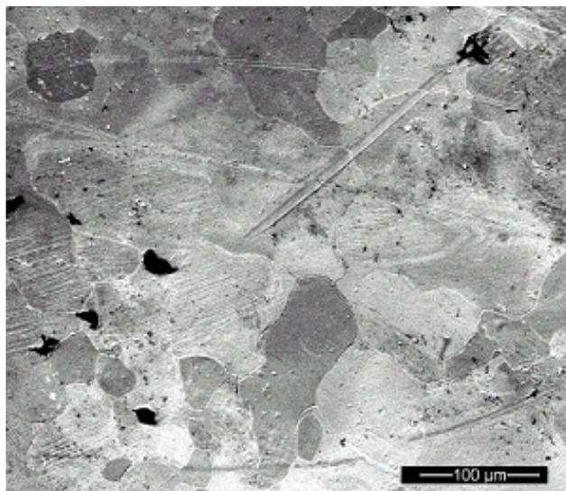
Fig. 1. Pd cold worked and annealed.
