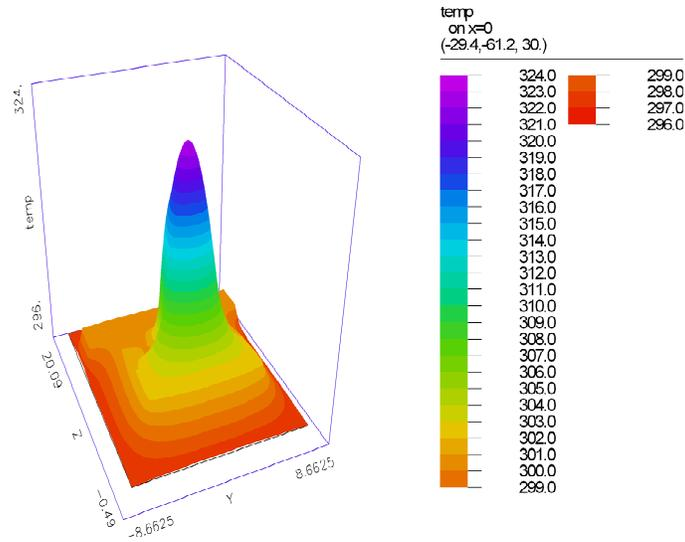
Fig. 3. Calculated 3-D Temperature distribution in the cell shown in Fig. 2.
